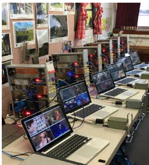
Figure 4: A group of six of the 12 laptop computers each streaming four high-definition videos via a Ngara point-multipoint link.
